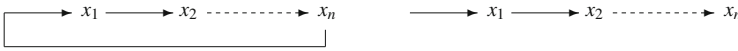
Fig. 2.2 A cyclic system ( left ), built by feedback from a cascade of n systems ( right )
